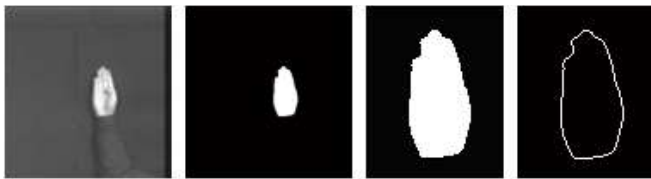
(a) alphabet b (b) segmented (c) resize (d) boundary Figure 4: Pre-processing of the gesture images
