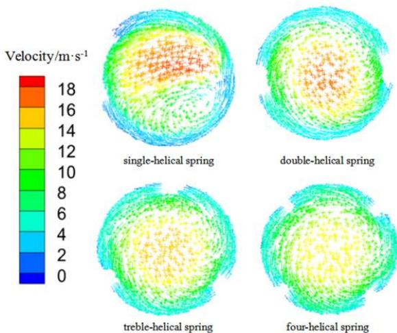
Fig.5 Velocity vector distribution of radial section at  $y=480\text{mm}$
