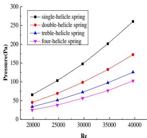
Fig.11 Comparison of heat exchange tube pressure drop
