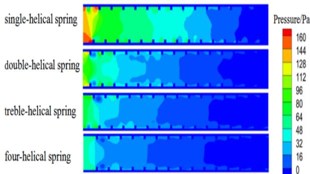
Fig.8 Pressure contour plot of axial section at  $x=0\text{mm}$
