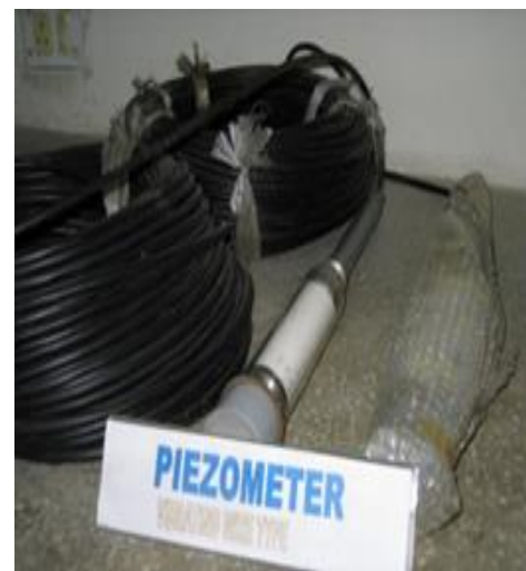
Fig 5-Vibrating Wire Piezometer in CSMRS
