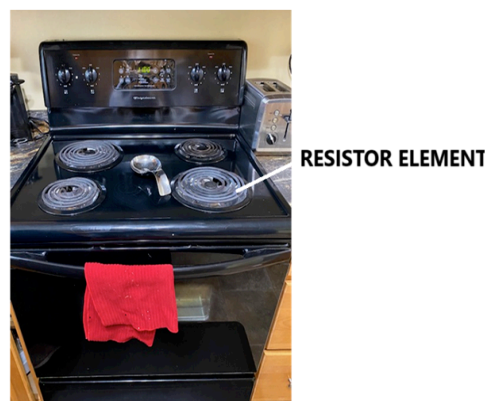
FIG 4 COOKING ON ELECTRIC STOVE WITH RESISTOR ELEMENTS
