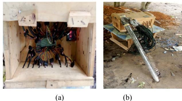
**Figure 6 :** Data acquisition system designed: a) inside the case; b) complete system
