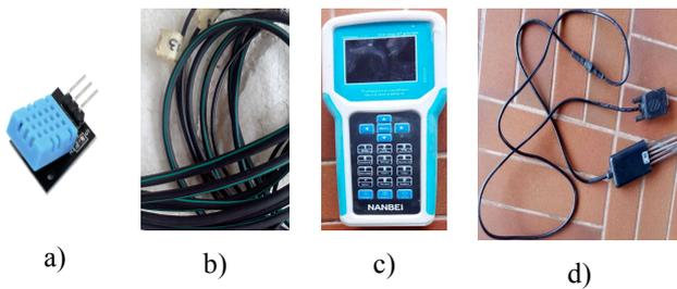
**Figure 4 :** Ground and air sensors: a) DHT11; b) 2×0.22 mm microphone cable; c) soil tester model JXBS-3001-SCY-PT; d) soil tester sensor JXBS-3001-SCY-PT
