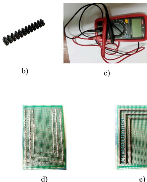
Figure 3 : Printed circuit board and its components: a) electronic components; b) 10 mm<sup>2</sup> 10 Amp electrical dominos; c) multimeter; d) and e) printed circuit board after soldering of female leads and resistors.
