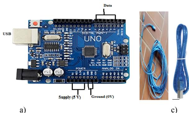
Figure 2 : Arduino Uno board and ports used: a) Arduino Uno board; b) printer cable
