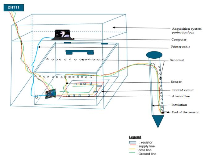
**Figure 7 :** Schematic diagram of the data acquisition system operating principle
