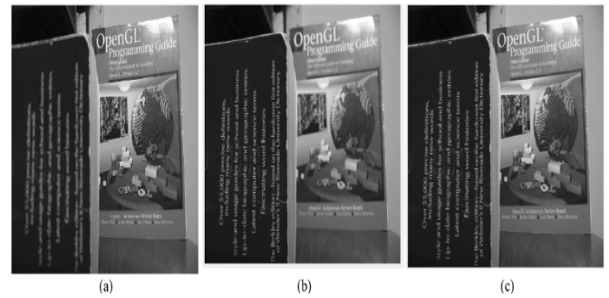
Figure 7: Examples of IF in photography domain. a) Back-focus Image b) Fore-focus image c) Fused image
